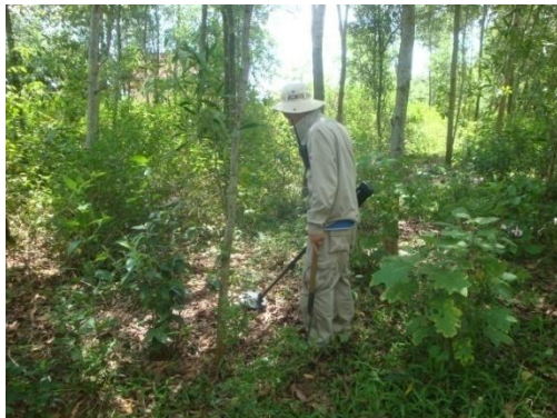
Technical survey using a handheld metal detector to identify defined hazardous areas. Removing safe land from the need for clearance reduces time and costs.
